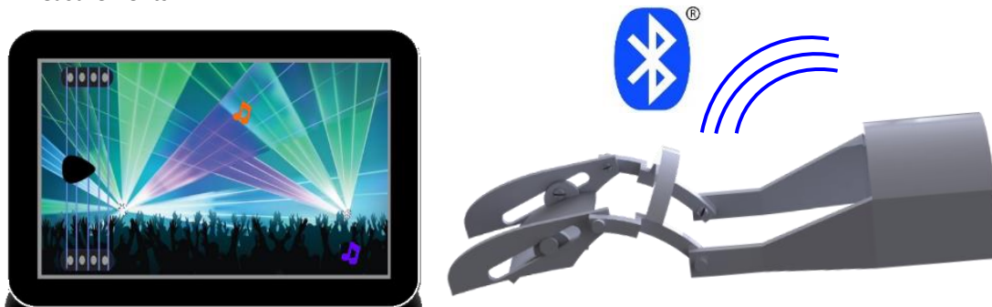
Figure 1. Therapeutic wrist exoskeleton connected via Bluetooth to a tablet that contains therapeutic games.
